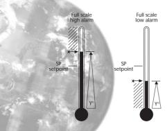
**dV.hi** sets off alarm signal when temperature rises above a pre-set temperature above the setpoint.
