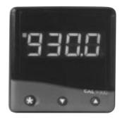
The CAL 3300 1/32 DIN and the CAL 9300 1/16 DIN miniature controllers share the same PID control strategy and features while giving the user the flexibility of a choice of panel format. Control can be optimised with a single shot autotune either on initial warm-up or at setpoint. A second setpoint can be configured in a variety of alarm modes or PID Heat-Cool strategy. A programmer offers a single ramp to setpoint with a choice of timed soak period before switching off the output.
