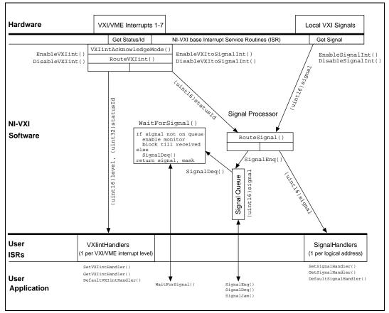
Figure 3-3 provides a graphical overview of the NI-VXI interrupt and signal functions.
