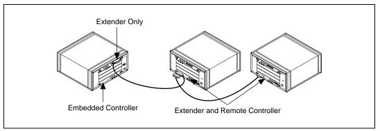
Figure 2-1. An Embedded Controller Connected to Other Frames via Mainframe Extenders Using MXI-2
