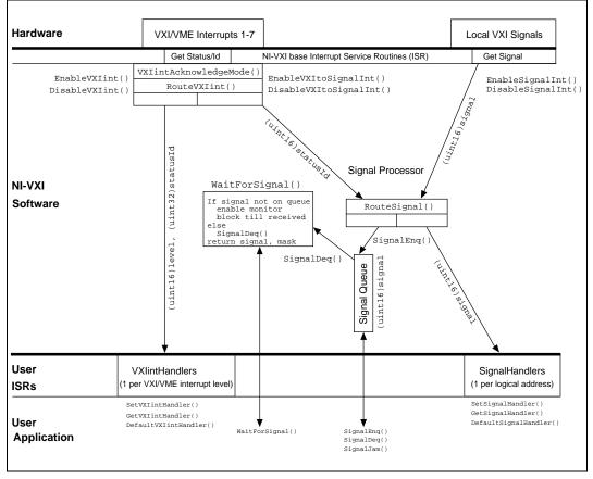
Figure 3-4. NI-VXI Interrupt and Signal Model
