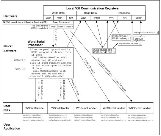
Figure 3-2. NI-VXI Servant Word Serial Model
