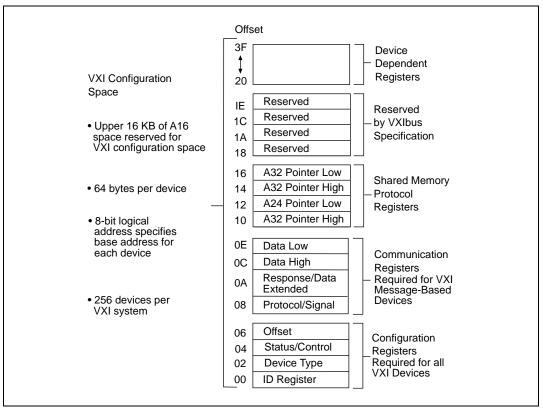
Figure 1-1. VXI Configuration Registers
