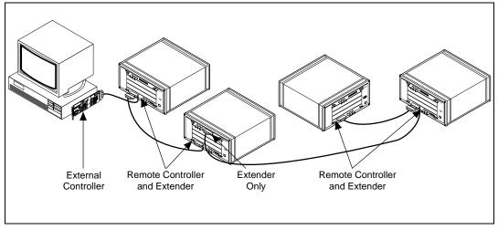
Figure 2-2. An External Controller Connected Using MXI-2 to a Number of Remote Controllers
