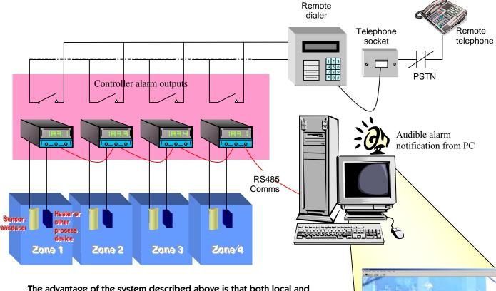
The advantage of the system described above is that both local and remote alarm notification can be configured so that an engineer can be informed of an alarm whether he is on or off-site.
