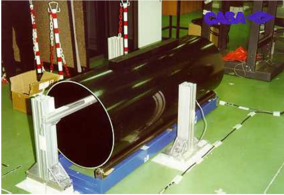
Figure 5 Prototype of the SCT detector support cylinder constructed in Spain.
