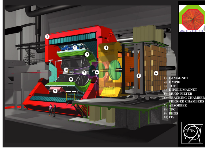
Figure 21. The ALICE detector layout
