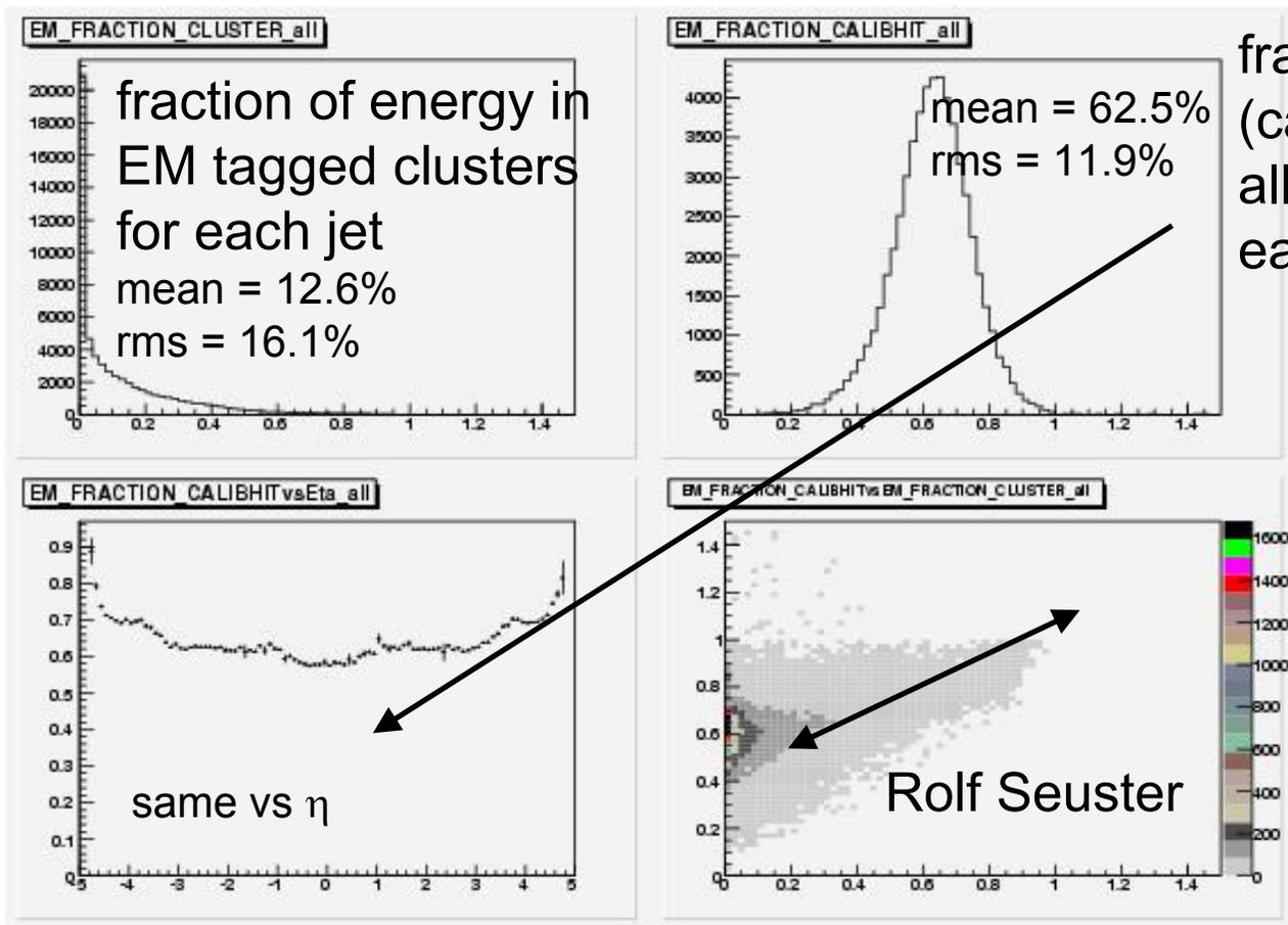
fraction of EM energy (calib hits) deposited in all cells of all clusters for each jet
