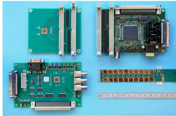
Figure 2.9: Printed circuits for ABCN25 ASIC testing. Top left and right: probe card compatible single chip board and driver PCB. Bottom left: single chip test card. Bottom right: 20 chip hybrid.
