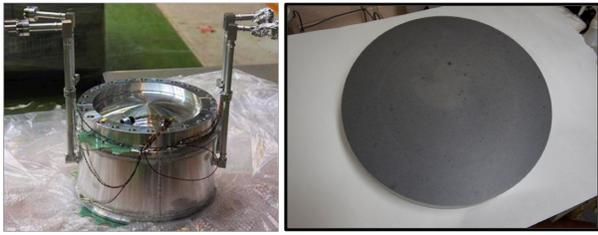
Figure 5: LH<sub>2</sub> absorber (left) and LiH disk (right).
