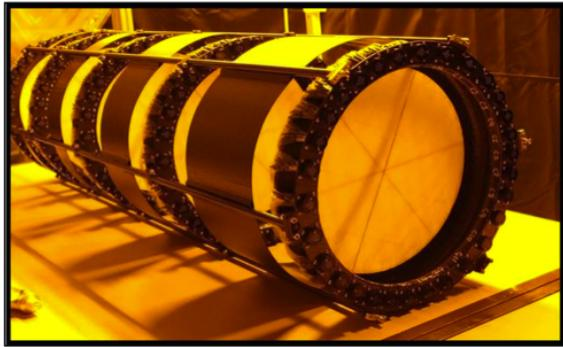
Figure 6: Photo of a scintillating fiber tracker.
