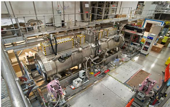
Figure 3: MICE spectrometer solenoids magnets installed in the experimental hall. The AFC module can be seen situated between the two solenoid modules.
