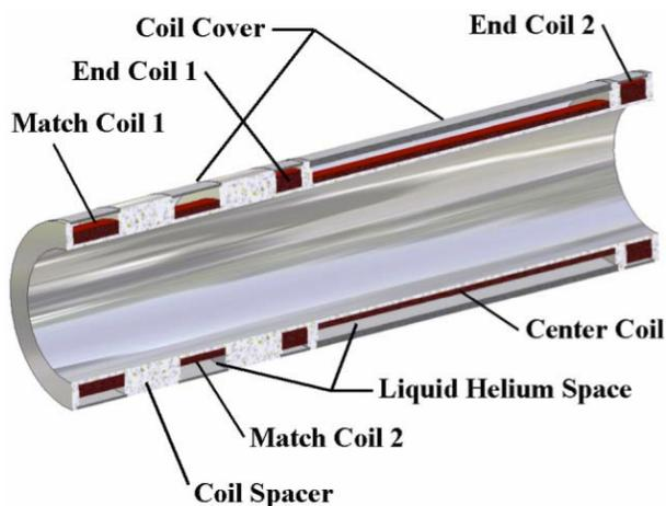
Figure 2: Cross section of a spectrometer solenoid magnet.
