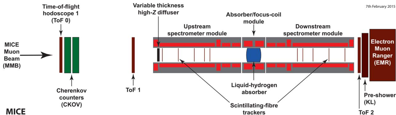
Figure 1: Schematic layout of MICE Step IV.
