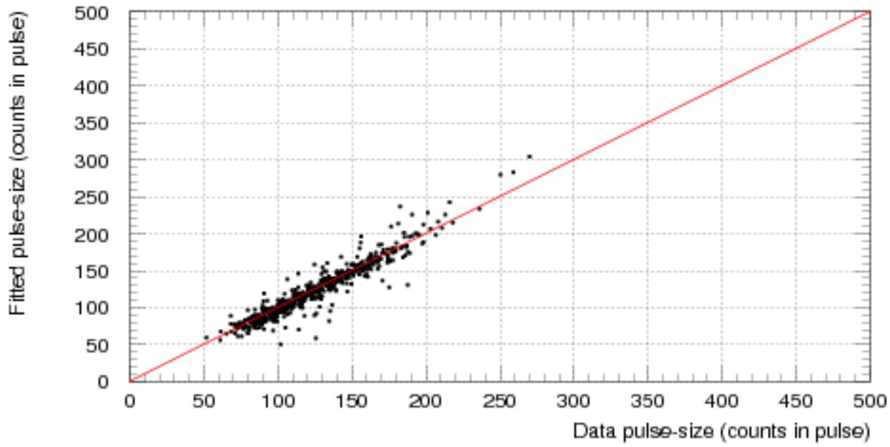
MUV1: fit compared with raw data; size, amplitude
